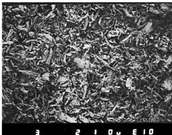
Fig. 1. SEM figure of the studied birch plywood grindings (magnification 32.5 \times ).
